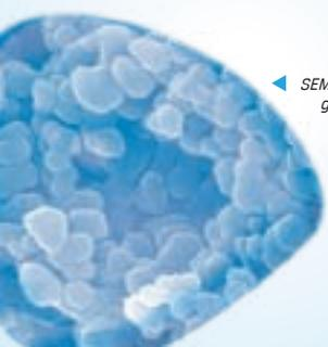
◀ SEM image focusing on the  $\gamma$ -alumina layer of a ceramic nanofiltration membrane
