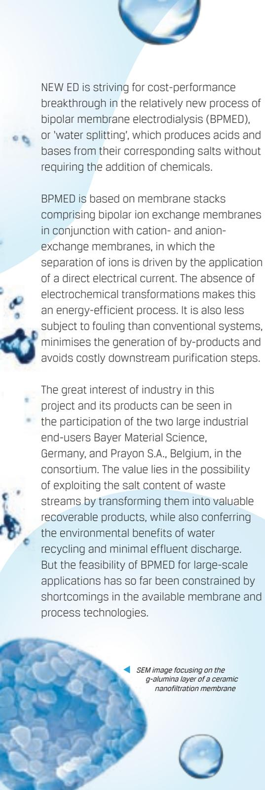
NEW ED is striving for cost-performance breakthrough in the relatively new process of bipolar membrane electro dialysis (BPMED), or 'water splitting', which produces acids and bases from their corresponding salts without requiring the addition of chemicals.
